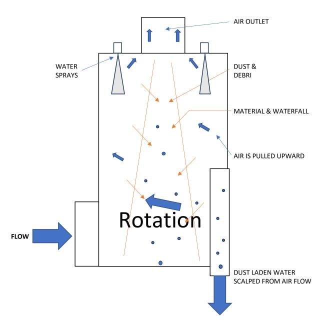
As the heavily particulate laden air is pulled upward through the Englo Tower Extractor, the particulate is forced to contact the water droplets from the tower's spray nozzles, causing it to be weighted and fall to the bottom of the cylinder. From there the particulate and water, entrained in the air flow inside of the tower, is scalped off and exits the tower. The Wet-Tower is custom designed to allow flexibility in sizing for the required air volume of the system.
