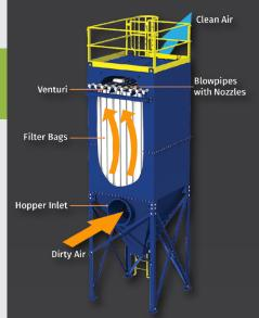
The TLM Baghouse operation is simple, proven, and efficient. Dust-laden air is drawn from the source through a duct system and into the hopper inlet.
