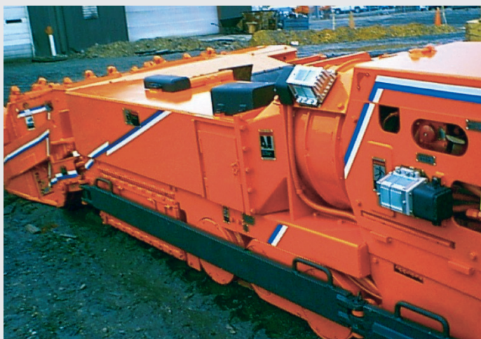
■ Englo Type 27 mounted on a Joy 14cm15 Continuous Miner—over 18,000 cfm
