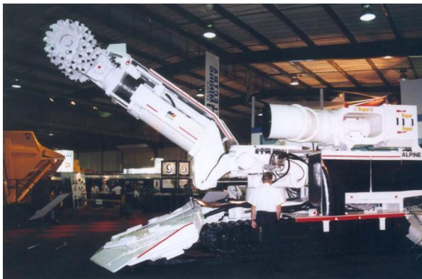
Figure 1-1 Equipment Mounted De-Duster
